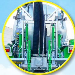
Hydraulic anti-drip system (Twist)
